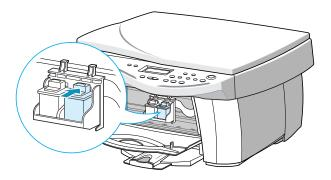
**8** After installing the print cartridges, close the cartridge door.
